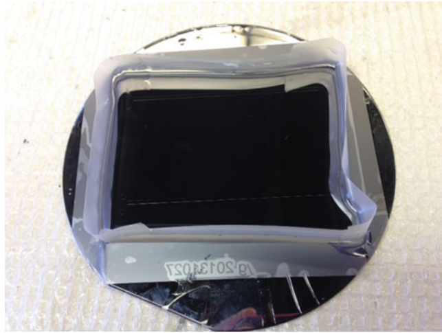
Fig. 3 To create a PDMS device, a mixture of PDMS and curing agent is poured over the exposed, developed, and processed wafer mold. A frame can be made around the wafer using scotch tape, and then PDMS is poured and allowed to cure at 95 °C for 1 h. The PDMS is then carefully removed from the wafer, cut to size, and any required holes are punched
