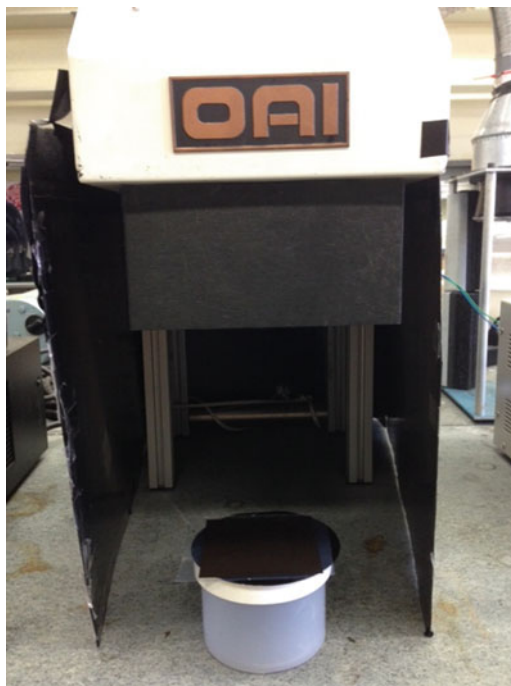
Fig. 2 A collimated UV light source is used to expose the photoresist through the mask. While a mask aligner can be used, for simpler devices the mask can be placed on the wafer and manually aligned. In this figure a 4" wafer was exposed through an affinity chip mask (see Fig. 1 for example). The exposure time depends on the light source power as well as the photoresist formulation and thickness
